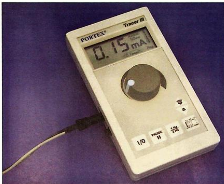
Figure 1.14 A peripheral nerve stimulator (reproduced with the kind permission of Smiths Medical)
