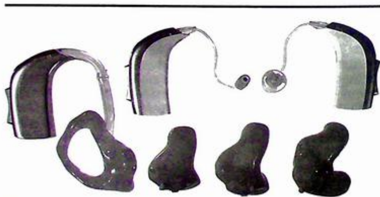
Figure 10-5. Hearing aid styles. Top: Behind-the-ear (BTE) hearing aid coupled to a custom earmold. BTE hearing aid with a receiver in the canal (RIC). BTE hearing aid with an RIC with a dome. Bottom: In-the-canal (ITC), half-shell in-the-ear (ITE), and full-shell ITE hearing aids. Reprinted with permission, Ryan McCreery.
