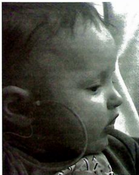
Figure 10-7. A probe microphone assembly used to measure the real ear or real-ear-to-coupler difference response from the ear canal. Reprinted with permission, Ryan McCreery.
