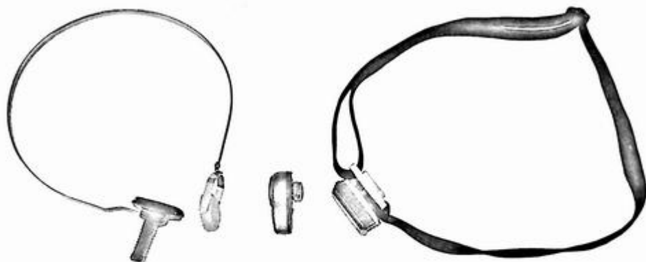
Figure 10-4. Coupling options for bone conduction devices. From left to right: (1) a hard bone conduction headband with an adapter for an osseointegrated auditory device processor; (2) an osseointegrated auditory device processor; (3) an osseointegrated auditory device processor coupled to a soft headband. Reprinted with permission, Ryan McCreery.
