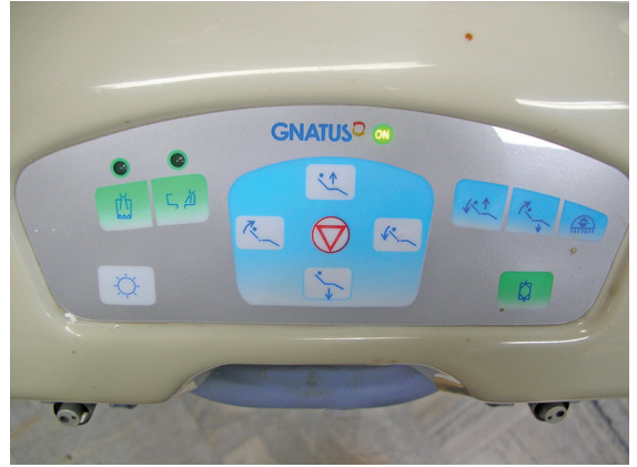
Figure 10.4 The front panel of the bracket table showing buttons for controlling the movement of the dental chair.
