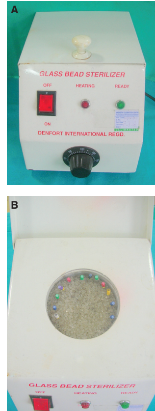
Figure 9.10 Glass bead steriliser. (A) Outside view. (B) Inside view showing glass beads.
