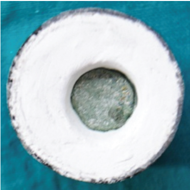
Figure 20.11 Solidified metal inside the casting ring, embedded in investment material.
