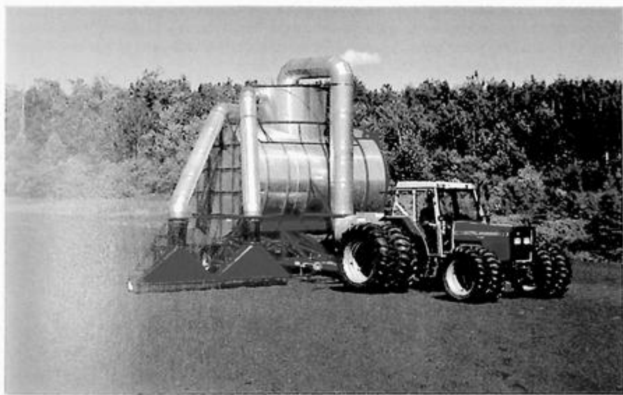
Figure 6-10 After preparation of the top layer of the bog for harvest, peat moss is harvested by this giant vacuum cleaner, and bagged for sale as a soil amendment. (Courtesy of Premier Tech)
