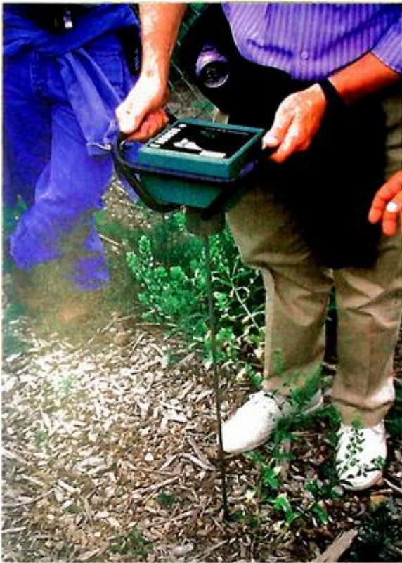
Figure 4-16 A digital cone penetrometer measures soil compaction in a habitat restoration project in Minnesota.
