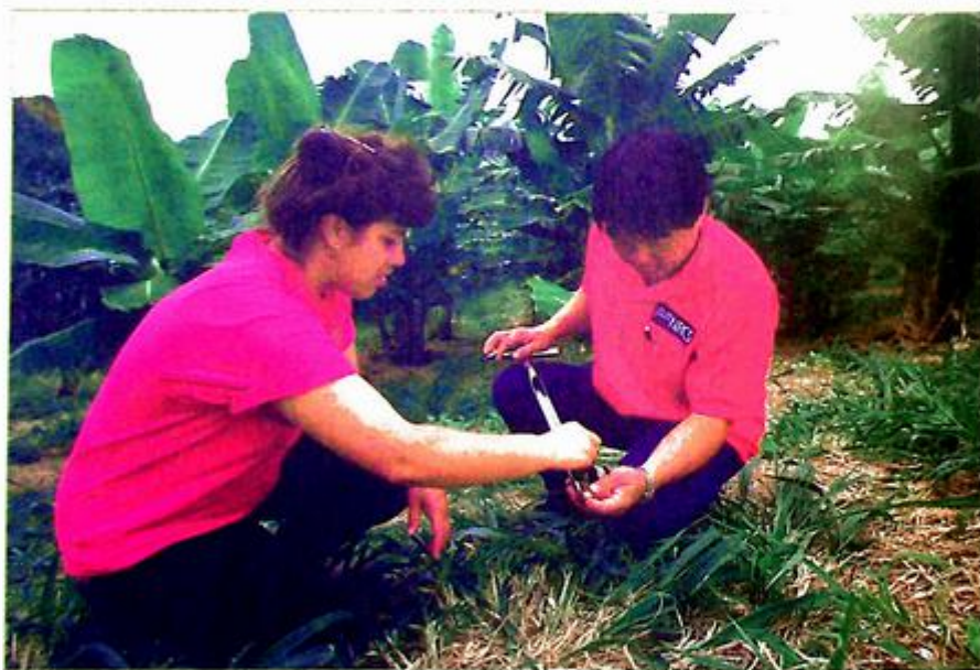
Using a probe to sample soil in a banana plantation in Hawaii. (Courtesy of USDA, Natural Resources Conservation Service)
