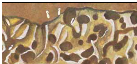
Fig. 118. Timber damaged by termites. Paper thin walls between runways creating a honeycomb. Photo©NSW Dept of Industry and Investment (E.H.Zeck).
