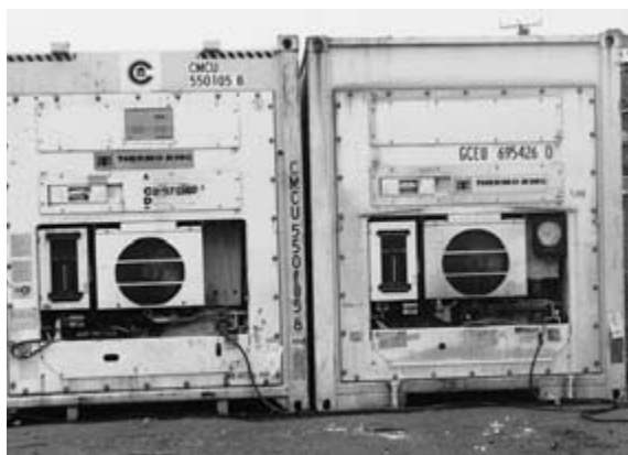
Figure 11.4 Packed controlled atmosphere reefer container plugged in to the mains electricity awaiting loading on the dockside in Castries, St Lucia, in 1998.
