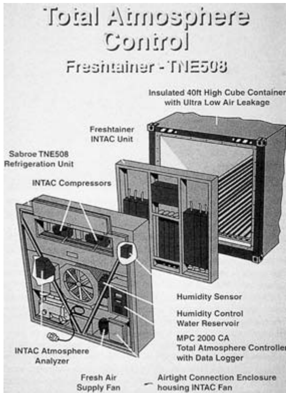
Figure 11.5 Diagram of a controlled atmosphere container (Freshtainer).
