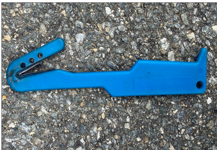
Photo 4-37. Ear tag removers are an efficient tool for runner removal (K. Orde).
