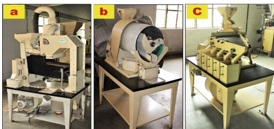
Fig. 6 Machine type used for vegetable seed processing. (a) Air screen cleaner, (b) Indented cylinder, (c) Specific gravity separator
