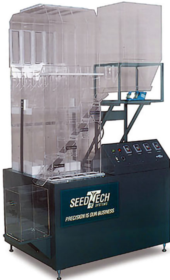
Fig. 5 Schematic diagram of pneumatic separator. (Source: https://www.usgr.com/seed-processing/wall-mount-air-seed-separators/ )
