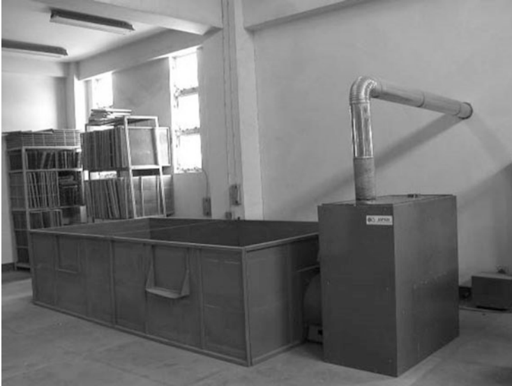
Fig. 1 Batch type hot-air dryer. (Photograph courtesy, Seed Processing Unit, IARI Regional Station, Karnal, India)
