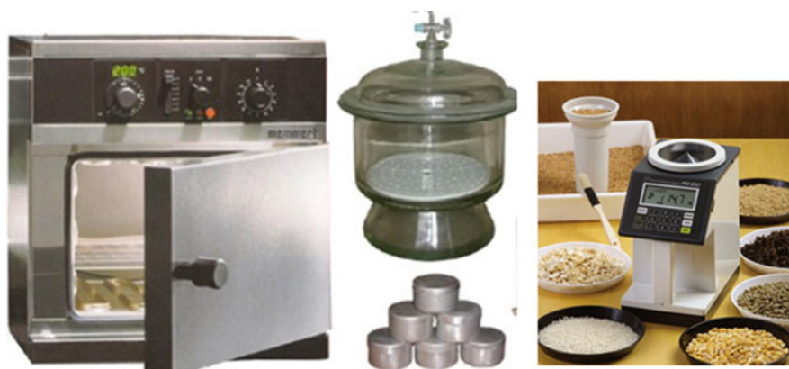
Fig. 4 Instruments for seed moisture determination (Source: A- theinstrumentguru.com/moisture-measurement ; B- directindustry.com )
