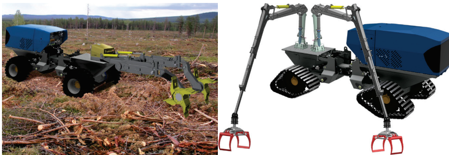
Figure 20. Visualization of continuous mounding conducted by the modular forest off road vehicle with attached Bracke Forest mounding arms (left), and visualization of the modular design with holistic options for machine design and testing (right). Photo: Sirius team 2017.
