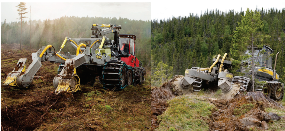
Figure 5. A Bracke two-row mounder (left) and Bracke two-row disc trencher (right). Photo: Bracke Forest AB.
