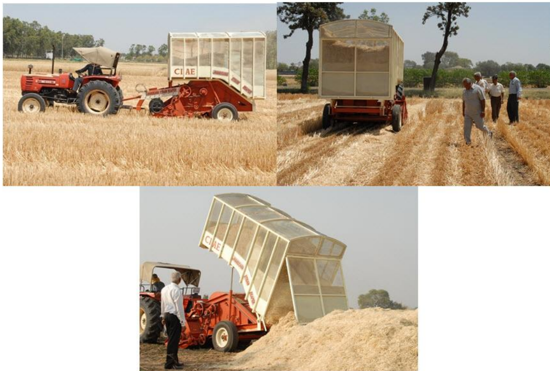
Fig. 3: Tractor operated straw reaper with storage box mounted above straw reaper.
