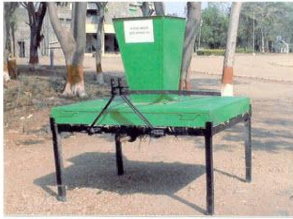
Fig. 5: Tractor mounted banana stem shredder.
