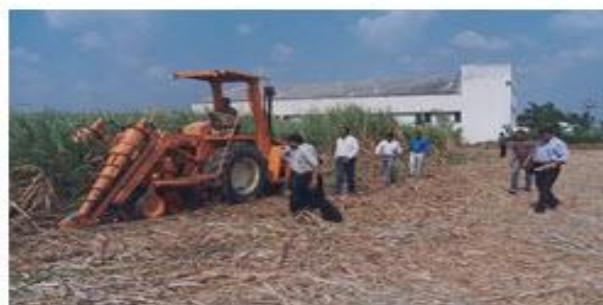
Fig. 3: CARIB (Barbadoes) cane cutter
