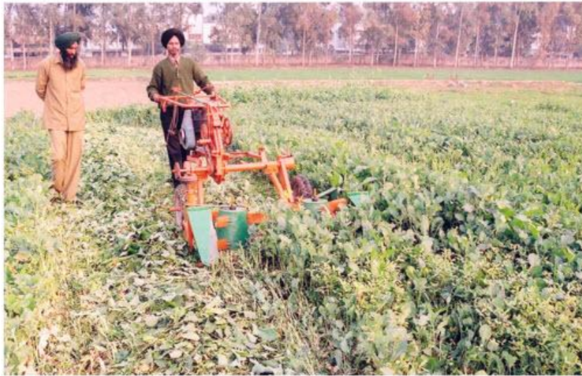
Fig. 5: Self-propelled fodder harvester (cutter bar type) in operation.
