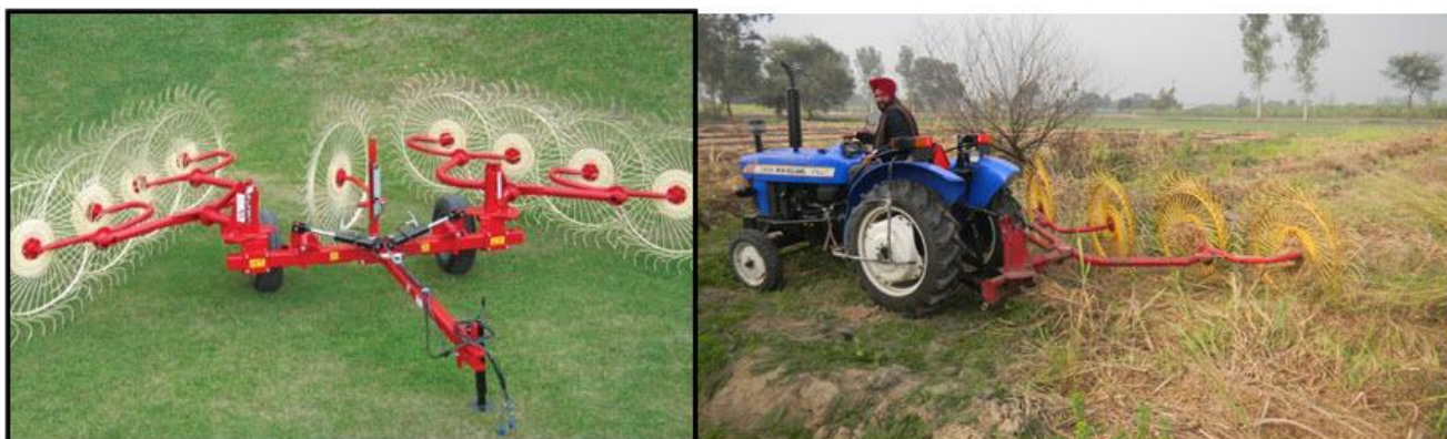
Fig. 14: A view of rakes used to collect cut hay or straw into windrows.
