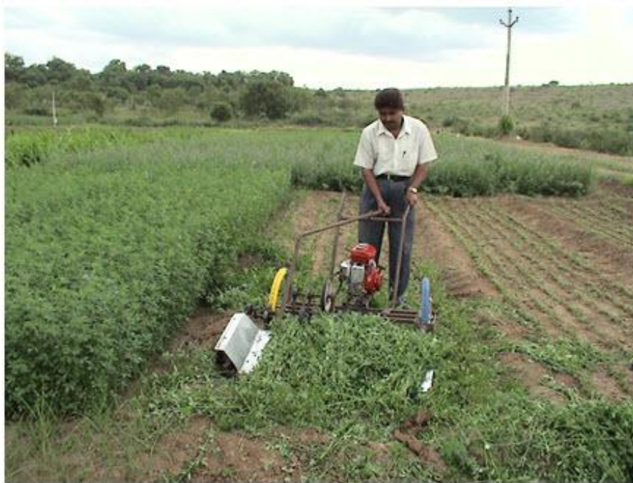
Fig. 6: A self-propelled lucerne harvester in operation.
