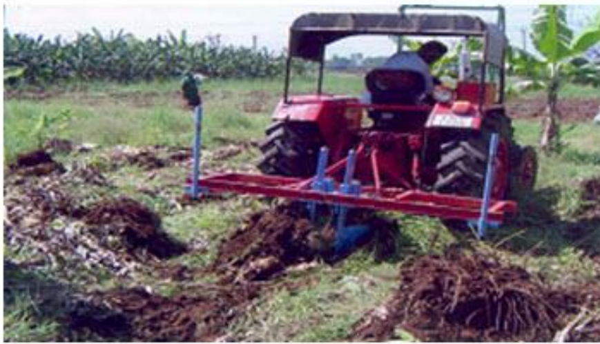
Fig. 7: Tractor mounted banana clump remover in operation.
