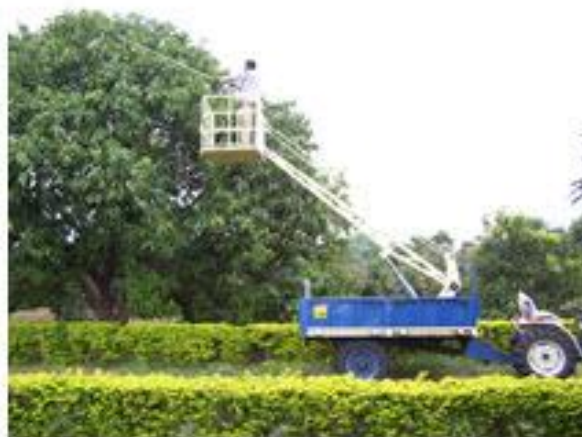
Fig. 4: Multi-utility elevator platform
