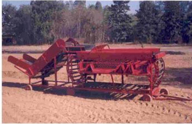
Fig. 1: Expanding pitch rubber spool potato sizer.
