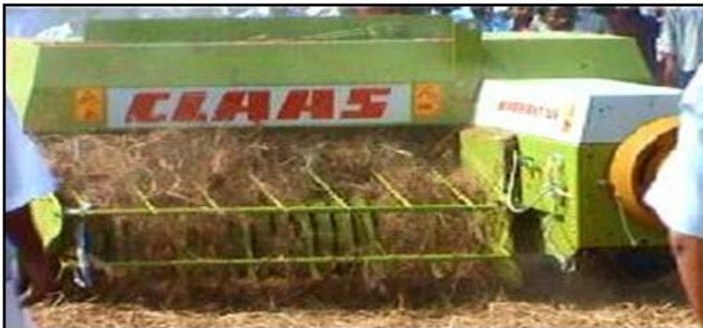
Fig. 7: Windrow pickup, conveying and feeding device.
