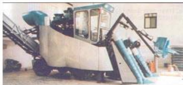
Fig. 2: VSI-RANE Sugarcane chopper combine harvester
