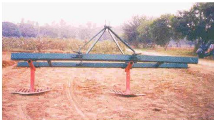
Fig. 2: Tractor-operated 2-row potato digger.
