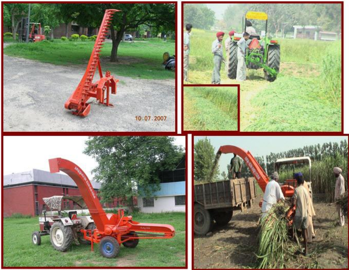
Fig. 4: Tractor operated cutter bar type forage harvester and loader.
