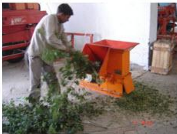
Fig. 6: Operation of plant shredder.
