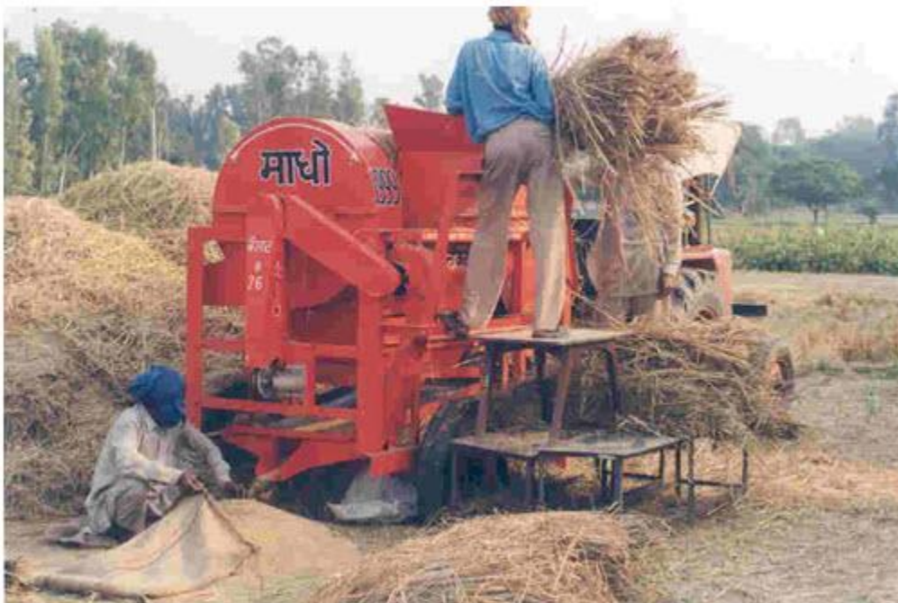
Fig. 8: Axial flow paddy thresher.
