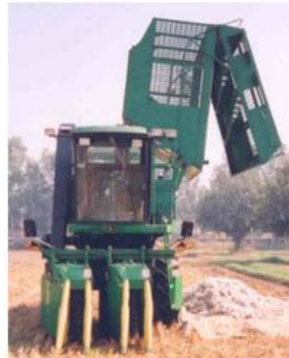
b) Unloading of mechanical picker
