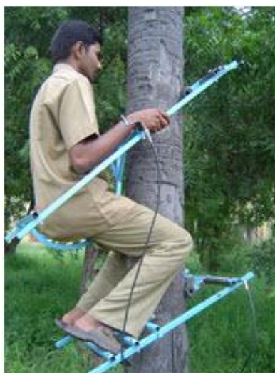
Fig. 2: Palmyra tree climber in operation
