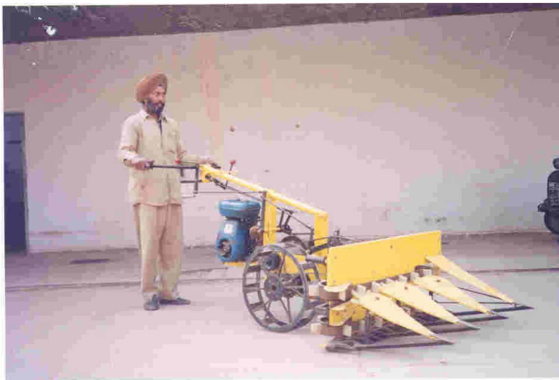
Fig. 4: Self-propelled vertical conveyer reaper-cum-windrower.
