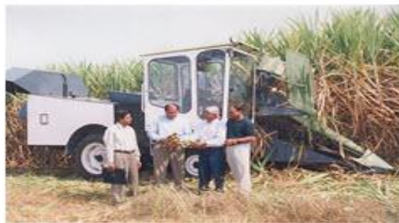
Fig. 1: VSI RANE whole cane sugar harvester
