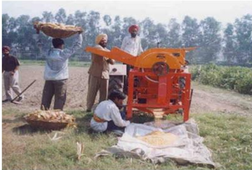
Fig. 3: Maize dehusker-sheller during operation.
