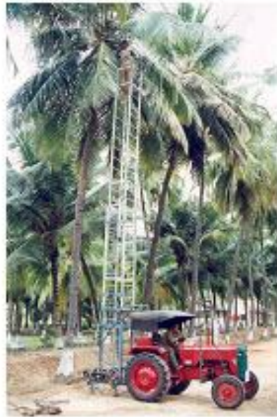
Fig. 5: Tractor mounted telescopic hoist
