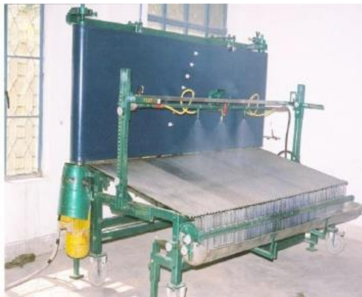
Figure 16.13 Boom sprayer test bench
