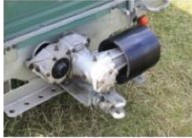
Figure 8.8 Belt pulley connected to tractor PTO
