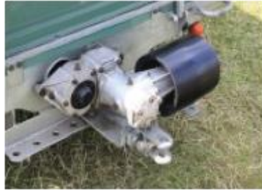
Figure 10.8 Belt pulley connected to tractor PTO
