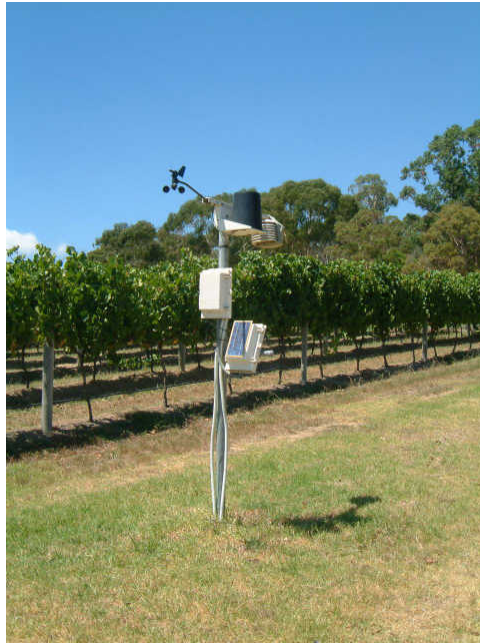
Solar-powered mini weather station in a Mornington Peninsular vineyard
