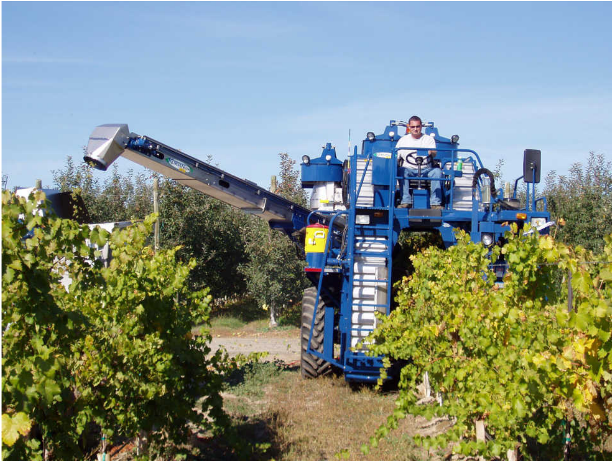
High-capacity grape harvester in one row, discharging into a gondola in the adjacent row
