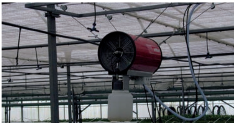
Figure 144. Static jet-transported hydro-pneumatic sprayer of ultra-low volume
