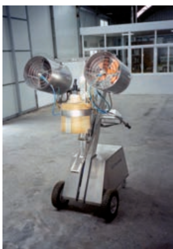
Figure 151. Manually adjustable hydro-pneumatic sprayer
