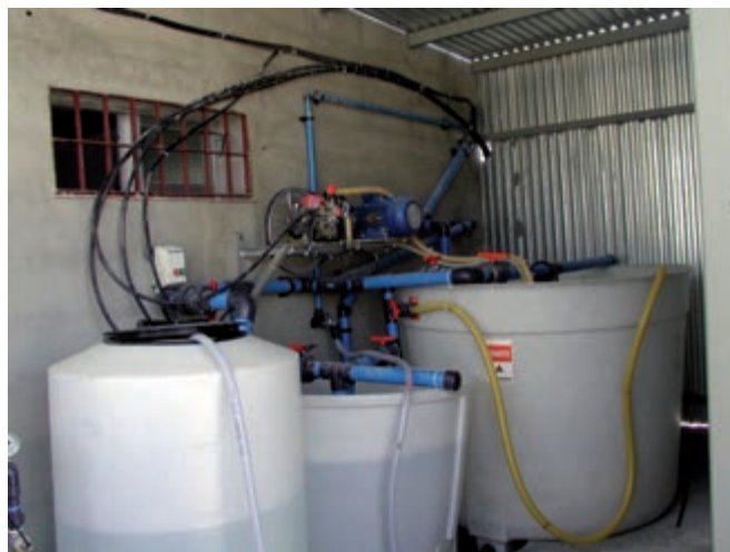
Figure 134. Tanks for phytosanitary treatments with a jet agitation system
