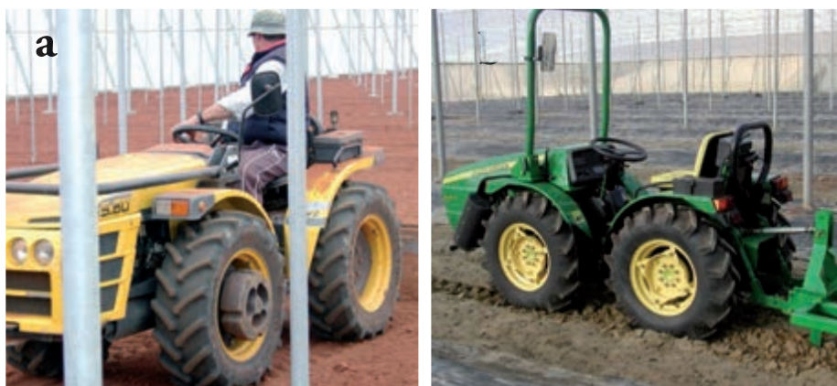
Figure 127. Four-wheel-drive articulated tractors used in greenhouses for the preparation of sand plots (a) and maintenance by ploughing (b)
