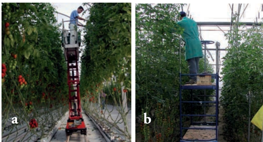
Figure 130. Lifting platforms for operators supported on heating rails (a) and on the ground (b)
