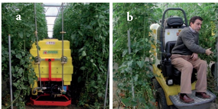
Figure 147. Self-propelled vehicles for hydraulic spraying: rear view of the treatment bar (a) and front view with driver seat (b)
