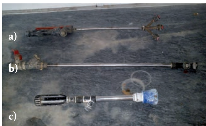
Figure 137. Spray guns for the application of phytosanitary treatments connected to a fixed network with three nozzles (a), two nozzles (b), and a single nozzle (c)
