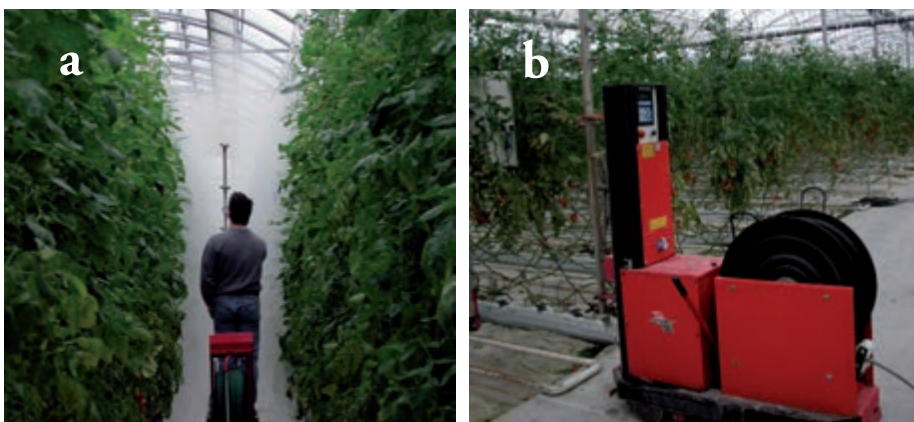
Figure 141. Self-propelled electric carts with vertical treatment bars: operator controlled, demonstrating the application of only water (a), and automated (b)
