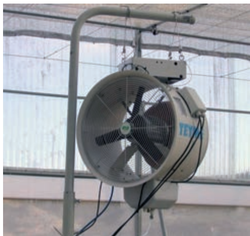
Figure 145. Centrifugal-pneumatic transported-jet sprayer
