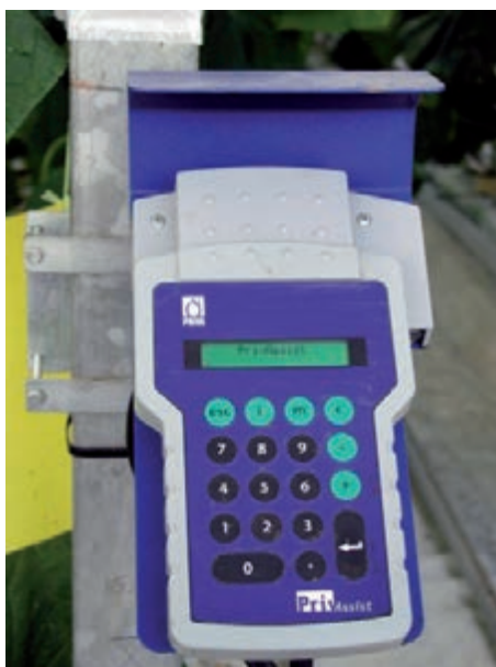
Figure 133. Electronic data storage system used to control time spent on field work
