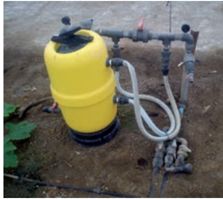
Figure 117. Fertiliser tank connected in parallel to the irrigation network
