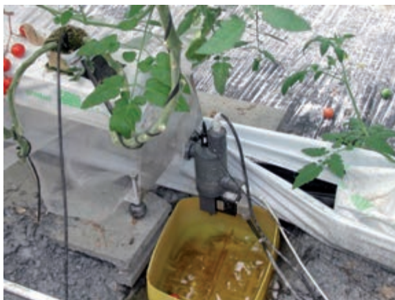
Figure 125. pH and EC sensors used for irrigation control in greenhouses
