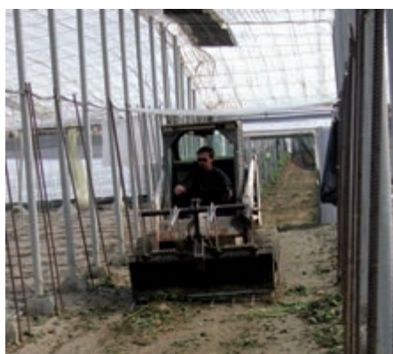
Figure 128. Shovel loader used in greenhouses for waste management
