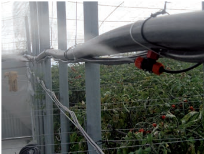
Figure 143. Stream of air and treatment drops generated by a fogging nozzle
