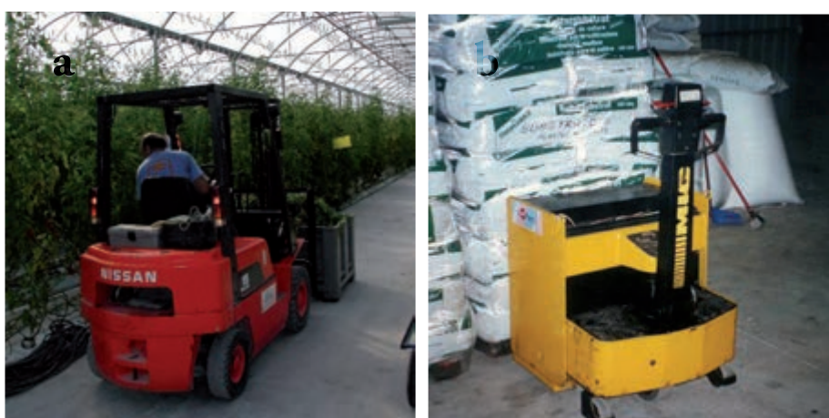
Figure 129. Forklift (a) and pallet jack (b) used for loading work and transport within greenhouses and nurseries
