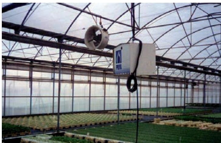
Figure 113. Measuring box with CO 2 concentration sensor
