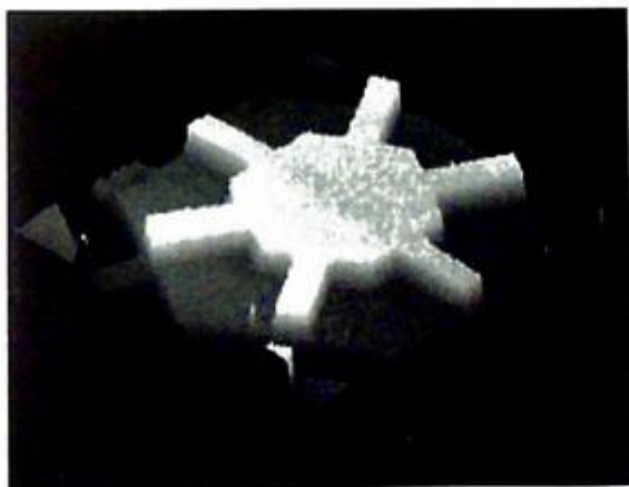
Atomic Force Microscope (AFM) image of one of thousands of cells on the surface of a Silicon Ultrasound transducer
