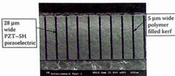
FIGURE 3.4 An electron micrograph of a 2-2 composite consisting of PZT 5H piezoceramics separated by polymer.
