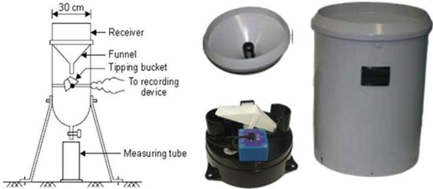
Fig. 9.2 Tipping bucket rain gauge
