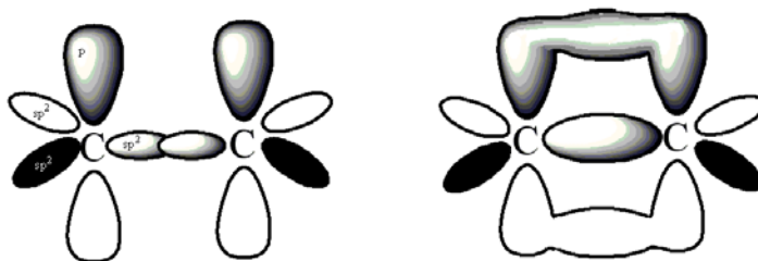
Figure 2-1. Formation of a \sigma and a \pi -bond between two sp^2 hybridized carbon atoms. The p -orbital has two lobes, one above and one below the C-atom.
