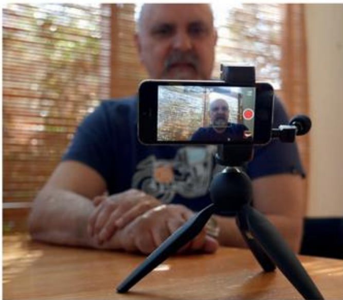
Figure 4.11 Ivo recording a selfie standup with smartphone fixed to Manfrotto Pixi using a Shoulderpod S1. Ivo Burum
