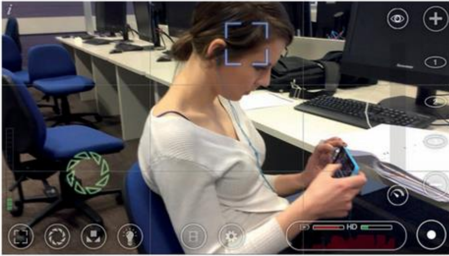
Figure 4.4 Filmic Pro screen showing the independent exposure ring and focus square. Ivo Burum
