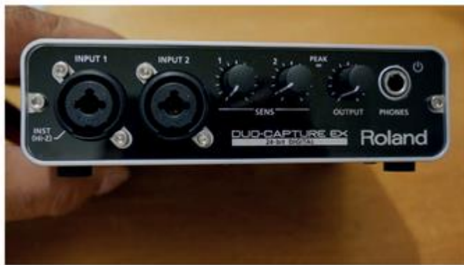
Figure 4.6 Using an interface device will enable multi-track recording as long as you record on multi-track device.
