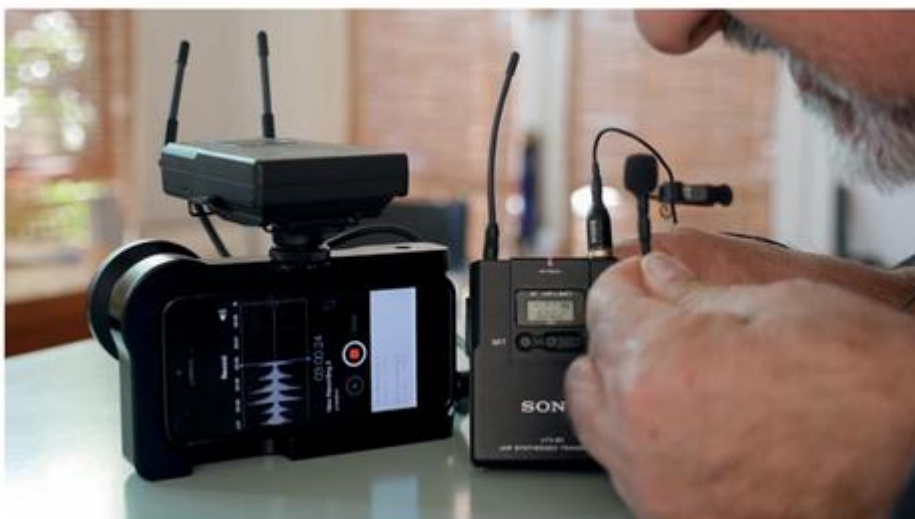
Figure 6.5 Testing the Sony UWP-D11 Radio Microphones for mojo work using a smartphone and mCAMLite. Ivo Burum
