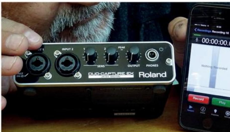
Figure 6.7 Roland Duo Capture EX two-track mixer interface next to a smartphone to show its compact size. Ivo Burum
