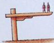
A cantilever is like a beam held only at one end
