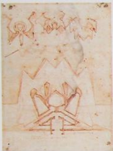
Michelangelo's Study of Fortifications Number 27 model the walls as sculpted surfaces. Regulating lines that suggest cones of vision (and angles of gunfire) provide the geometric underpinning for the overlay of thickened lines whose bistré infill registers the
