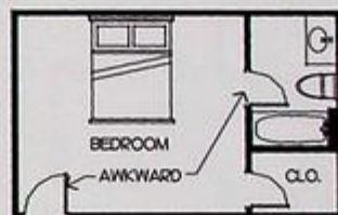
BAD DOOR ARRANGEMENT
