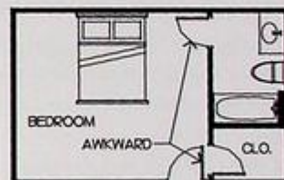
ANOTHER BAD DOOR ARRANGEMENT
