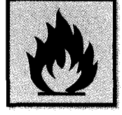
f fire hazards
