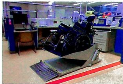
Figure 13.8 Motorized wheelchair lift, allowing the patient to remain in the chair during dental treatment.
