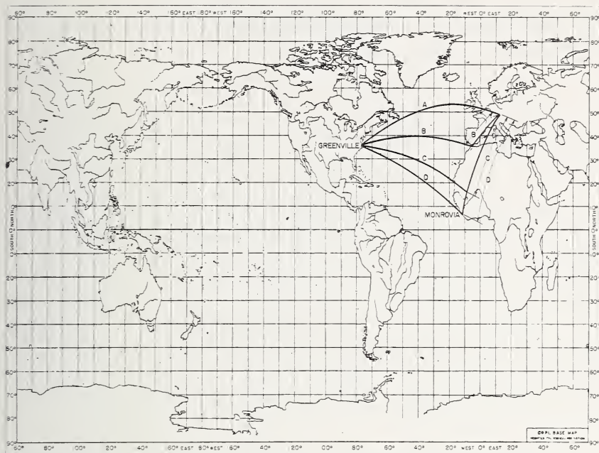
FIGURE 4.25. Transmission from Europe to the United States via side-scatter over Africa.
