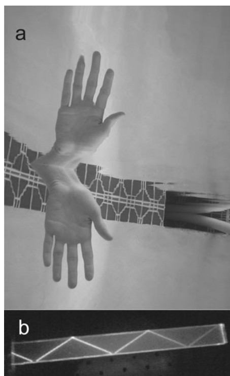
Figure 10.9.2 a: The hand's image is reflected by the underside of the water, due to total internal reflection. (Image courtesy of and © Jacob J. Loman) b: A laser beam bounces inside a block of the plastic PMMA, due to total internal reflection. (Image from Wikimedia Commons.)
