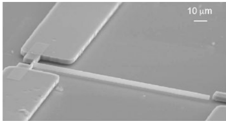
Figure 3.4.1 A micromachined silicon cantilever used to detect the pressure or molecular weight of gas via the change in the oscillation frequency due to damping. The cantilever is produced by a combination of photolithography and etching (“micromachining”) and is suspended a few \mu\text{m} above the substrate, so that it can oscillate in a plane parallel to the substrate, as shown in the schematic diagram. Top image reprinted with permission from Y. Xu, J. -T. Lin, B. W. Alphenaar, and R. S. Keynton, Appl. Phys. Lett. 88 , 143513 (2006). Copyright 2006, American Institute of Physics.
