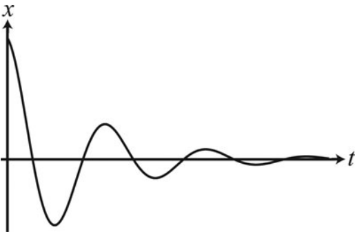
Figure 1.1.2 Motion of a tree branch when pulled up and then released.
