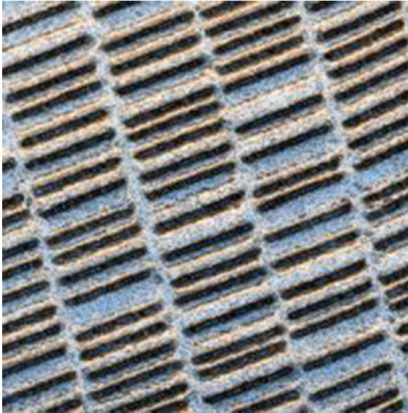
FIGURE 7.7 Magnetic force microscope image of the elongated magnetic nanoparticles on a hard drive layer.
