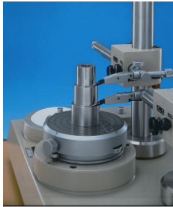
Figure 2.30. Significance of a parallelism (straight line/straight line) inspection (Mitutoyo Canada)
