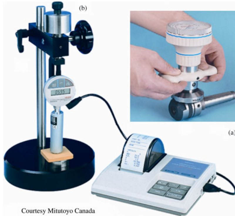
Figure 9.8. (continued) Barcol apparatus for measurement of the hardness of plastics, elastomers, and natural synthetics (rubber, acrylic, acetate resin, polyester, thermoplastic, PVC, and neoprene)
