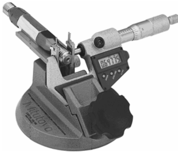
Figure 1.27. Measurement of pitch diameter (inches) using the wire method (Mitutoyo)
