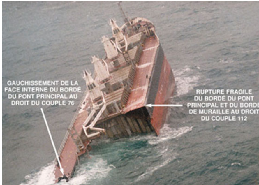
Figure 9.12. Aerial photo of the “FLARE” taken from the rear side (Source: Investigation report on a marine (excerpt), according to “Courrier technique” de l’OTUA n° 64, Breaking and sinking Bulk Carrier “FLARE” (Cabot Strait in January 16, 1998)
