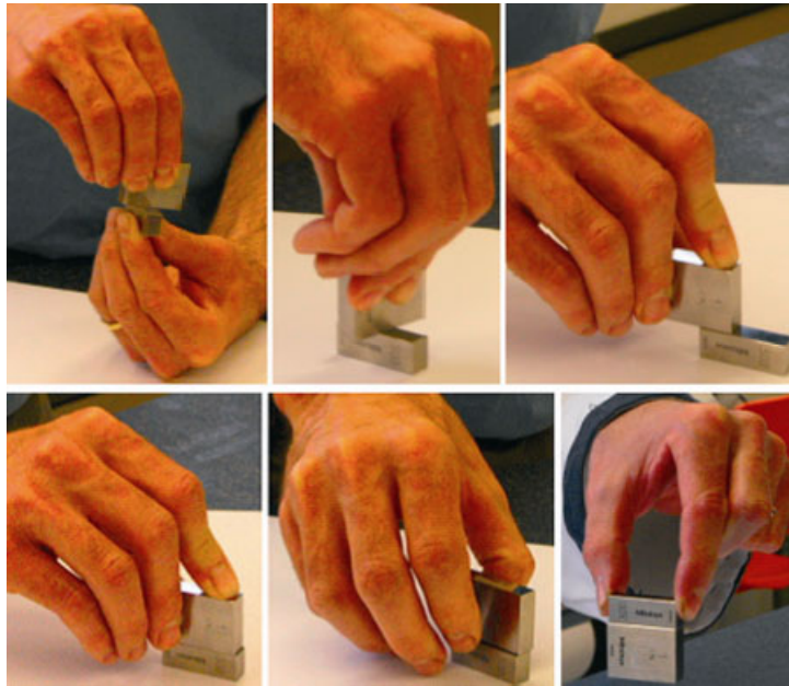
Figure 3.6. Explanatory steps for blocks adhesion
