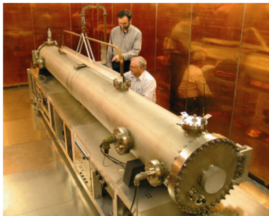
Figure 3.2. Atomic clock INMS (source: NRC, Ottawa, Canada). Model of a clock (CsV) in Cesium, built by the NRC in Ottawa (Canada). In the photo Mr. Rob Douglass (crouching) and Jean-Simon Boulanger, NRC, Ottawa. Frequency and Time Research Group, NRC-INMS
