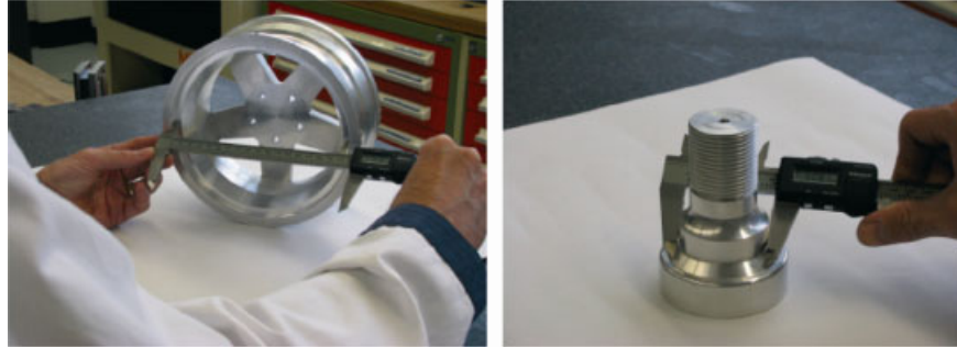
Figure 3.44. Reading inner and outer diameters
