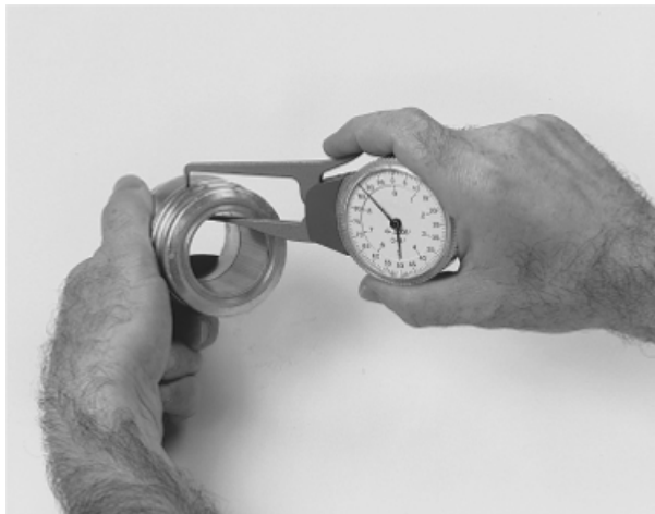
Figure 3.18. Comparator with probe arm for outer measurement (courtesy Mitutoyo)
