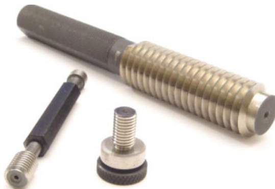
Figure 8.23. Ring and plug gauge for easy control of ISO thread
