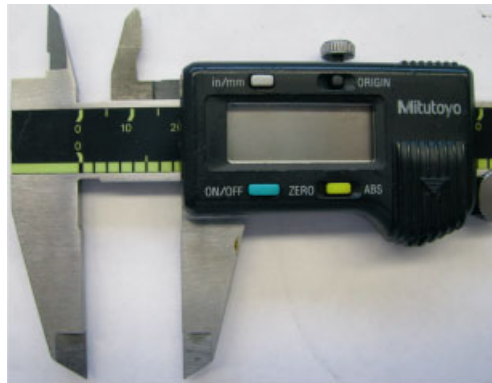
Figure 3.46. Photograph of damaged vernier with offset beaks
