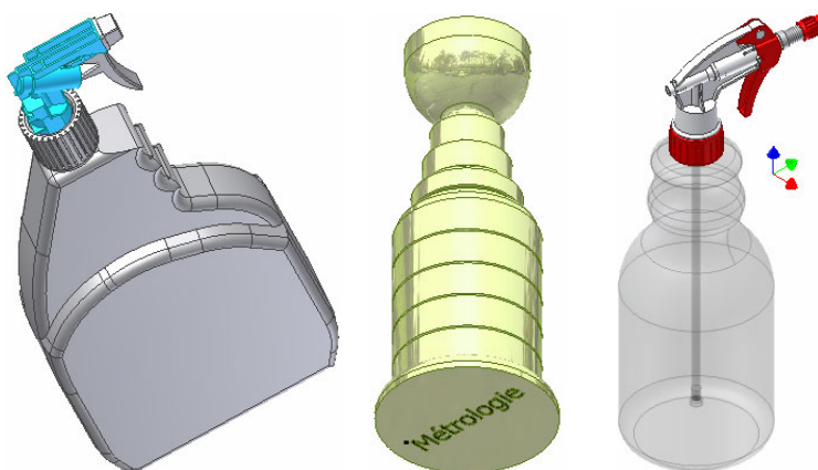
Figure 7.4. Representation of hybrid models: solid + surfaces in Inventor Pro
