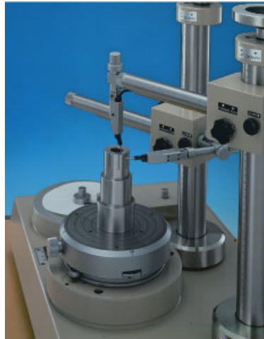
Figure 2.37. Control of the concentricity (coaxiality) by mechanical comparison (Mitutoyo)
