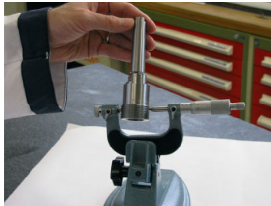
Figure 3.59. Measurement of pitch diameter by screw thread micrometer
