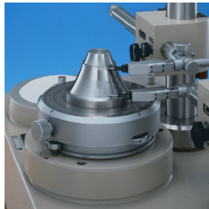
Figure 2.54. Interpretation of a cone form tolerancing (courtesy of Mitutoyo)
