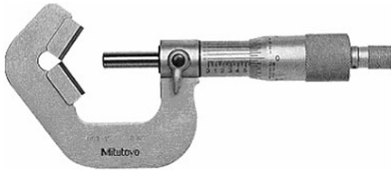
Figure 3.68. V-shaped outside micrometer for angle inspection (courtesy of Mitutoyo)
