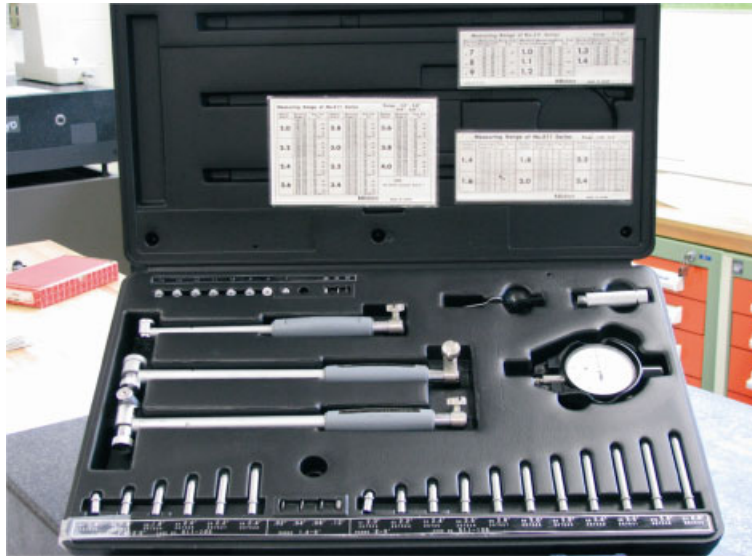
Figure 3.30. Mounting kit for telescopic bore gauge (see Table A2.1)
