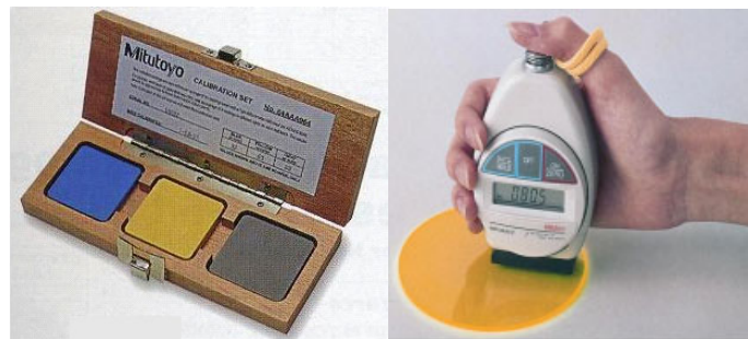
Figure 9.9. Standard etalons for Shore hardness for plastics; portable Shore durometer (Mitutoyo)
