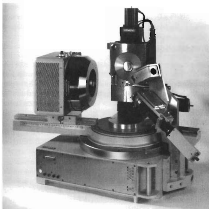
Figure 18.7 Siemens microdiffraction system shown with multiwire area detector, xyz stage, and video camera.
