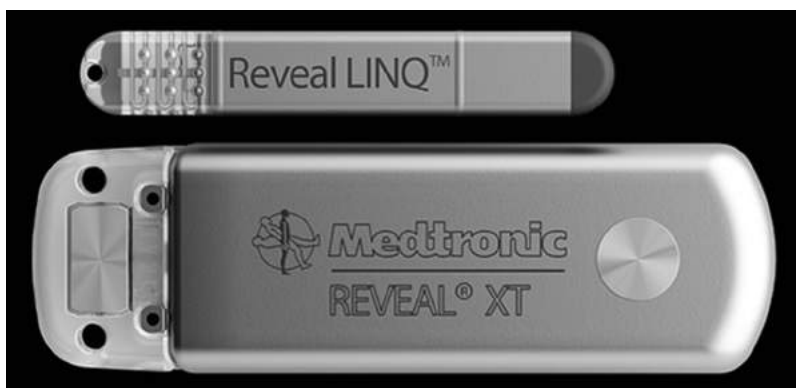
Fig. 6.2. Example of an older (lower image) and a more recent (upper image) generation implantable loop recorder (ILR). Note the more compact size of the newer ILR.
