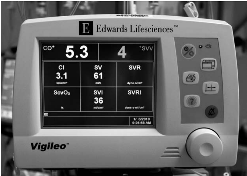
Figure 7.2 • The Edwards Vigileo FloTrac continuous cardiac output monitor which is connected to the arterial line.
