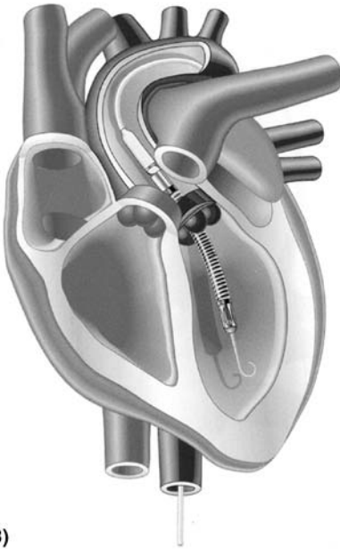
Figure 11.7 • The Impella devices. (A) The basic design of the catheter with an inlet that lies within the left ventricle and an outlet within the ascending aorta, next to which is located the rotary pump. (B) The Impella 2.5 device (12 Fr diameter) and Impella 5 (21 Fr diameter) devices have similar designs and are placed percutaneously to lie across the aortic valve. (C) The Impella LD device is placed through a graft sewn to the ascending aorta.
