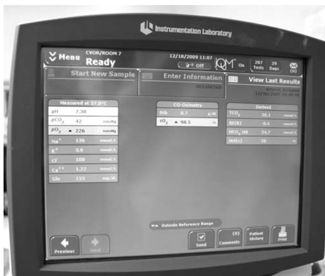
Figure 5.10 • Point-of-care testing machine available to the perfusionist to obtain arterial blood gases, electrolytes, glucose levels, oxygen saturations, and hematocrit levels.
