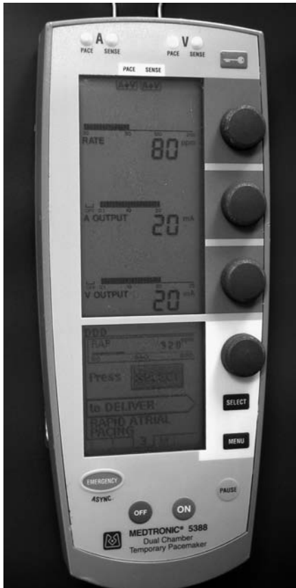
Figure 11.16 • The Medtronic model 5388 external pacemaker. This device can be used to provide pacing in a variety of modes, including AAI, DVI, DDD, and VVI pacing. It also has rapid atrial pacing capabilities.
