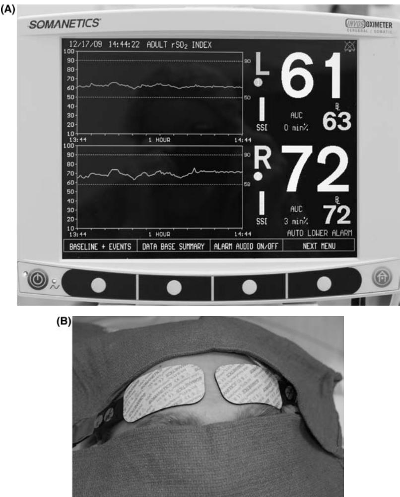
Figure 4.10 • (A) The Somanetics INVOS cerebral oximeter. This device uses near-infrared spectroscopy to measure the regional saturation of predominantly venous blood directly in the brain through optical sensors placed on the right and left sides of the forehead (B).
