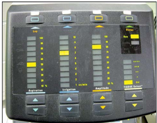
Figure 10.6: CUSA: Showing the adjustment of amplitude, irrigation, suction and tissue select modes
