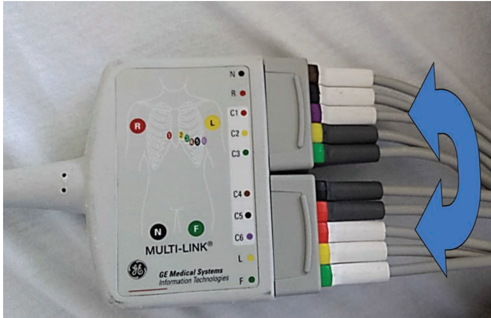
Figure 16.2.2 Inversion of the connections (note the colors which do not match up).
