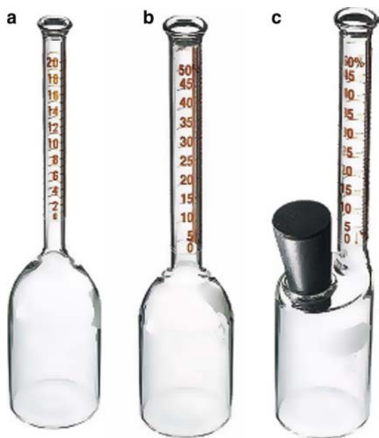
8-6 figure Babcock milk test bottles for milk (a), cream (b), and cheese (Paley bottle) (c) testing. (Courtesy of Kimble Glass Co., Vineland, NJ.)
