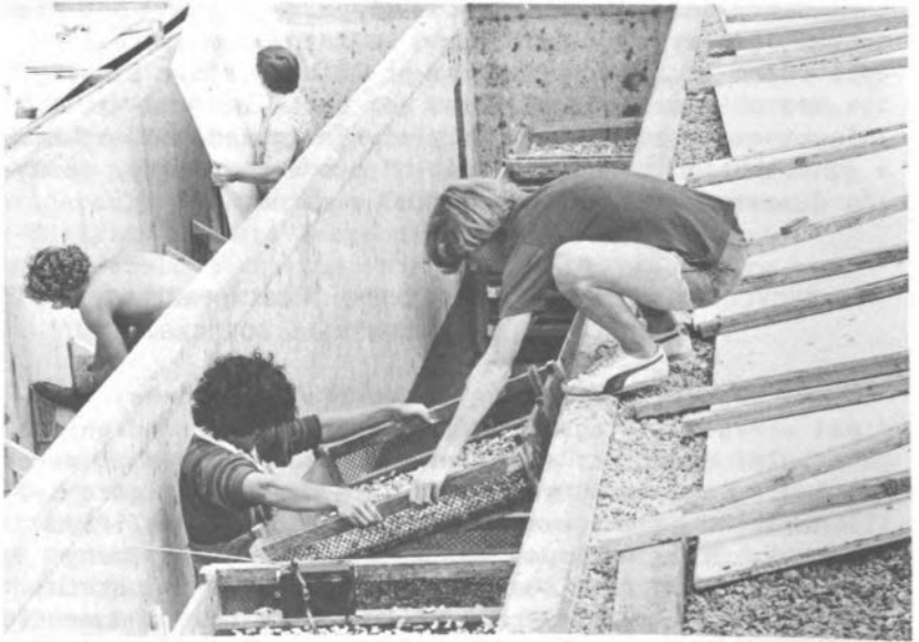
FIGURE 5-2 In this Woods Hole experiment, it was found that diluted inputs of treated sewage were an excellent nutrient supply for planktonic pond algae, which in turn provided the food supply of shellfish grown on racks in adjacent raceway enclosures. (Woods Hole Oceanographic Institution)
