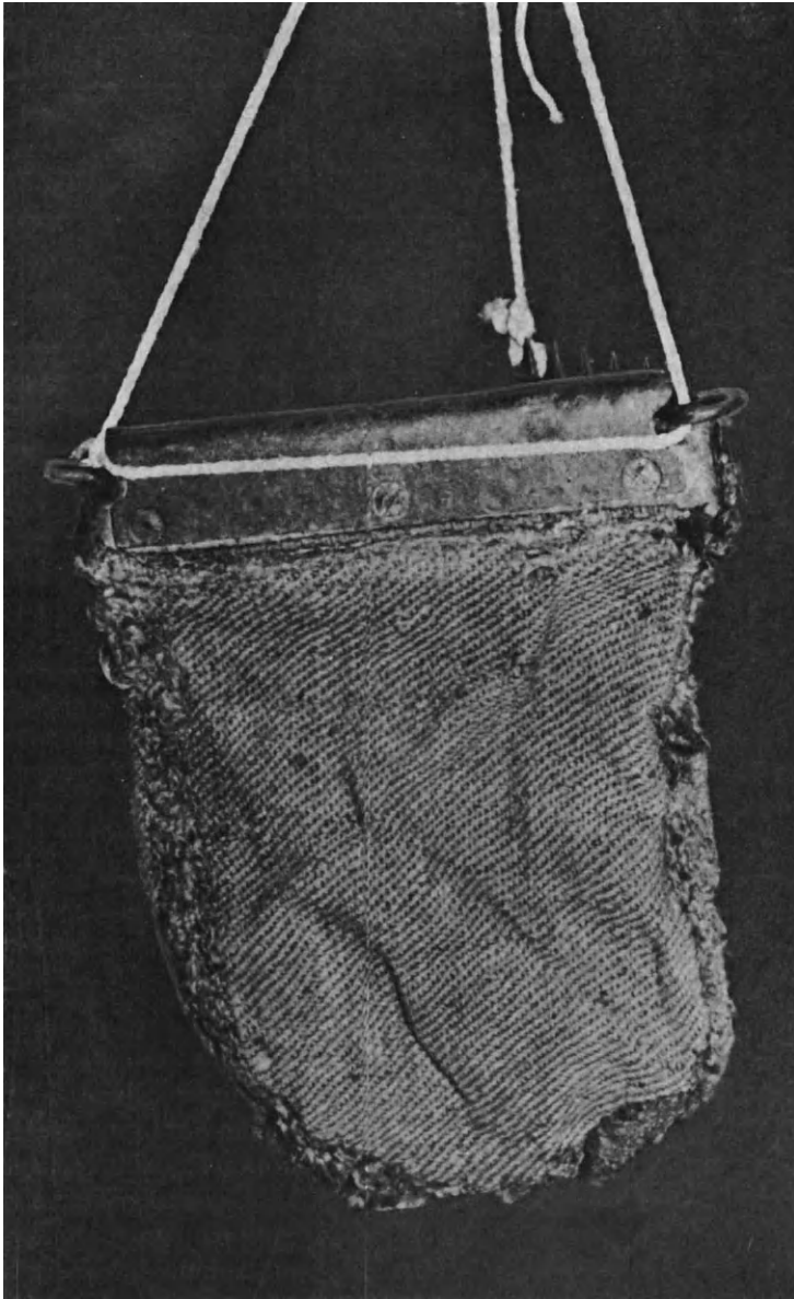
FIG. 51. Steinmann's dredge for investigation of the bottom.
