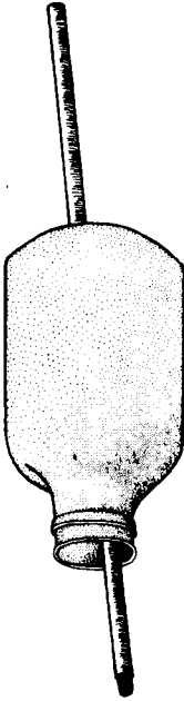
FIG. 72. Douglas's method for collecting epilithic algae. (Redrawn from Douglas, 1958.)
