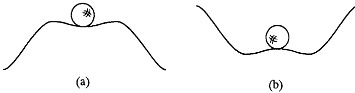
Figure 118 Limitations of a local stability criterion
