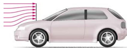
Flow past a car antenna is approximately two-dimensional, except near the top and bottom of the antenna.
