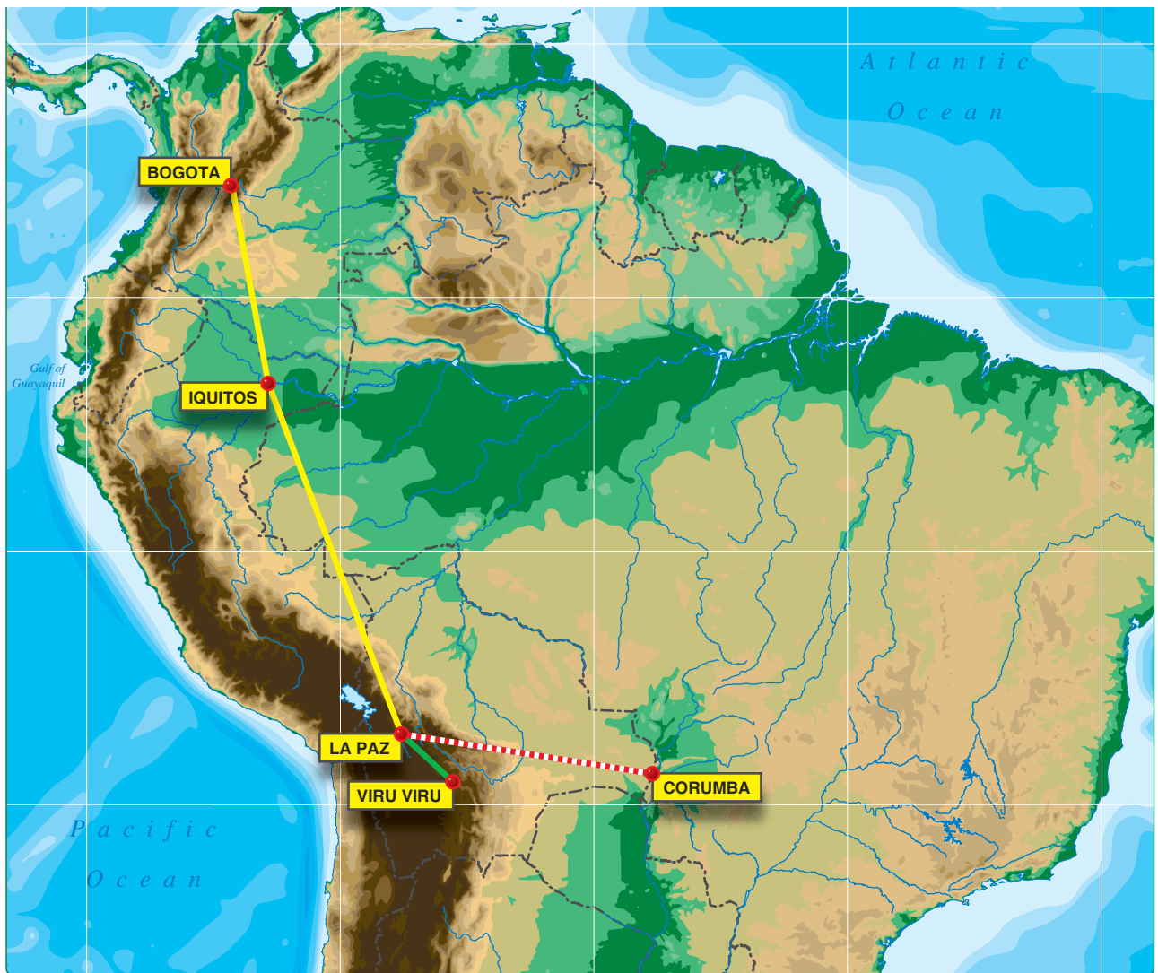
Figure 7-3. The pilots of a King Air 200 had a flight from Bogota, Colombia, to Iquitos, Peru, (for fuel) and then to La Paz, Bolivia, as final destination. They listed Viru Viru (located at Santa Cruz, Bolivia) as their alternate. The aircraft was equipped with a Bendix King KNS 660 that provided integrated navigation solutions based upon VOR, DME, and two variants of VLF radios. At that time, GPS had not yet been integrated into the FMS.
