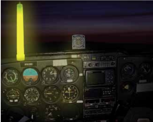
Figure 3-8. A chemical stick is useful to carry onboard the aircraft at night. It comes in various colors, intensities, and durations, and it provides ample illumination within the flight deck. This does not replace the regulatory requirement of carrying flashlights.
