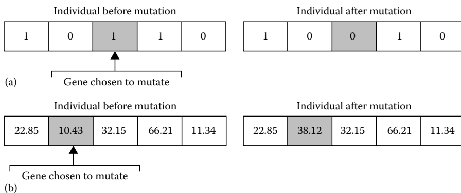
FIGURE 29.5 Scheme of simple mutation operator for individual with binary representation (a) and real-number representation (b).
