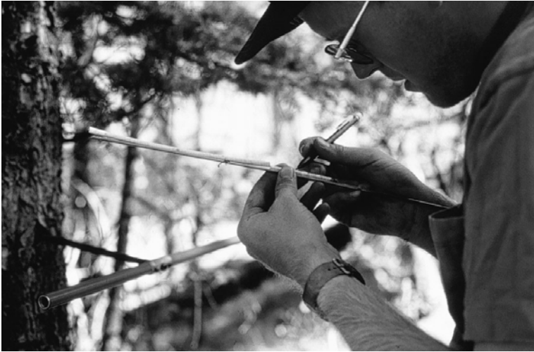
Figure 5.1 Using an increment borer to count rings and estimate the age of trees. Photo by Stephen DeStefano.
