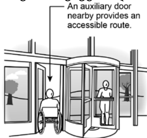
Auxiliary Door at Inaccessible Revolving Door
